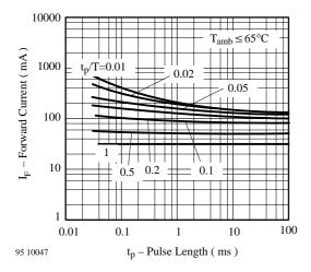
Figure 3 Forward Current vs. Pulse Length
