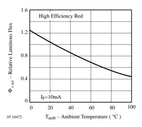
Figure 6 Rel. Luminous Flux vs. Ambient Temperature
