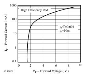
Figure 5 Forward Current vs. Forward Voltage
