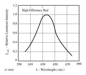
Figure 9 Relative Luminous Intensity vs. Wavelength
